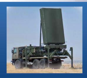
The MR84 is a mobile S-Band Multi-Role Radar (MR) Family implementing an advanced 3D Active Electronically Steered Array (AESA) supporting modular and scalable architecture.
