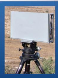
GR12/15 persistent ground and coastal surveillance radar is a new advanced high resolution radar with unique and outstanding capabilities. Featuring simultaneous multibeam technology, the radar provides persistent surveillance and instantaneous target tracking over a wide area.
